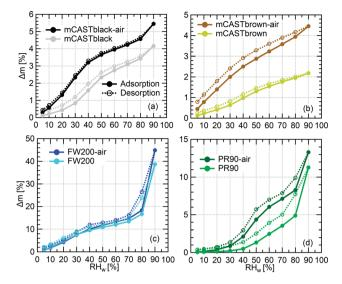
Fig. 7 Dynamic water vapour sorption (DVS) isotherms for fresh and synthetic air  $(N_2 + O_2)$  oven-heated (300 °C) soot. The solid lines with closed symbols and dashed lines with open symbols indicate adsorption and desorption isotherms, respectively. Each isotherm loop represents for an individual measurement. Note different y-axis scales.
