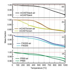
Fig. 4 TGA curves for fresh and oven-air-heated ( $N_2 + O_2$  atmosphere) bulk soot samples. Solid and dotted lines indicate two individual TGA runs. The T was held for 30 minutes at 300 °C. Red dashed line shows the bulk sample mass fraction benchmark, *i.e.*, 100%. Note the different y-axis scales for the samples.
