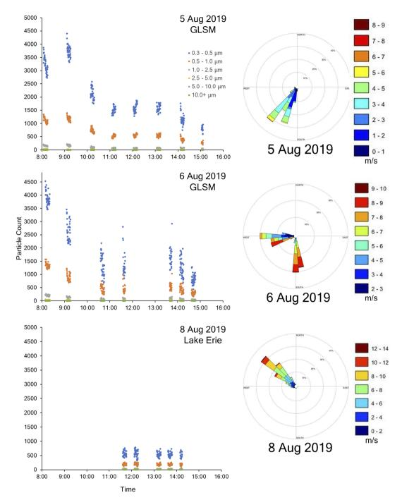
Fig. 5 Airborne particle counts over the course of the day. Data were recorded from a PMS7003 OPC onboard the AirDROPS. The first two graphs show flights that occurred August 5<sup>th</sup> to 6<sup>th</sup>, 2019 at GLSM while hovering 10 m over the water. The third graph depicts the flights on August 8th, 2019 while hovering 10 meters over the water at LE. To the right of each graph is the corresponding wind rose which shows wind direction and speed (m s<sup>-1</sup>) each day.
