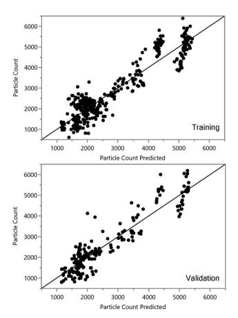
Fig. 8 Measured vs. predicted particle counts used in the best fit model. The graph on the top panel shows the fit of the model on the training set of data, while the graph on the bottom shows the fit of the validation set of data. The model was made using the wind speed, temperature, and wind direction through the JMP Pro neural network modeling. The model was trained on two days of collected data, and verified on a random subset of the collected data that was not used to train the model.
