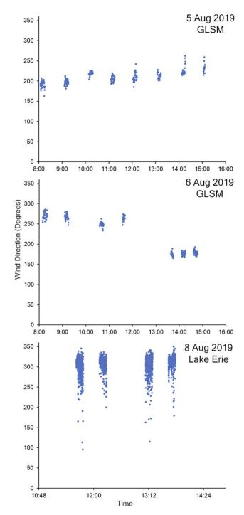
Fig. 3 Wind direction (degrees) over the course of the day. The first two graphs represent August  $5^{th}$  to  $6^{th}$ , 2019 at GLSM. The third graph represents August  $8^{th}$ , 2019 at LE. The wind direction was determined using a sonic anemometer for August  $5^{th}$  to  $7^{th}$ , 2019, and using GLOS data for August  $8^{th}$ , 2019.
