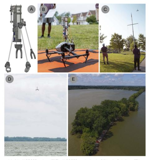
Fig. 1 (A) Engineering model of the AirDROPS package. (B) The AirDROPS attached to the DJI Inspire 2 platform. (C) Intercomparison flight of the AirDROPS adjacent to the sonic anemometer mounted on the flagpole. (D) Sampling mission at GLMS, 10 m above the surface of the water. (E) Drone image and aerial view of the sampling location at LE to the right of the point in the image.
