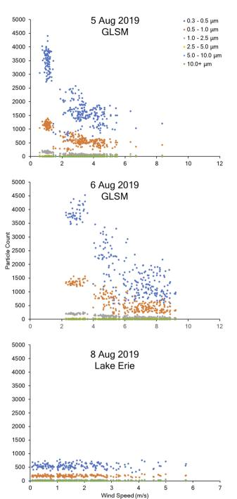
Fig. 6 Airborne particle counts recorded from the OPC onboard the AirDROPS, and windspeed from the sonic anemometer mounted on a flagpole and drone-modeled data for LE. The first two graphs show flights that occurred August  $5^{\rm th}$  to  $6^{\rm th}$ , 2019 at GLSM while hovering 10 m over the water. The third graph depicts the flights on August  $8^{\rm th}$ , 2019 while hovering 10 m over the water at LE.
