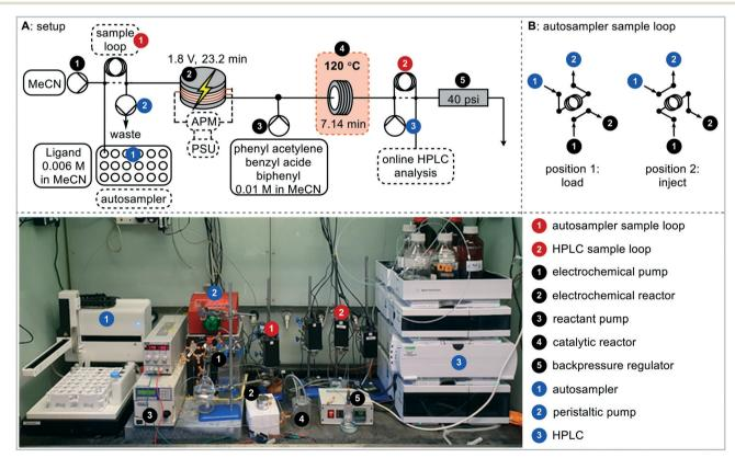
Fig. 5 A: Automated catalyst generation and activity screening. The platform generates in a stepwise fashion an array of catalysts through an electrochemical process followed by thermal reaction with online HPLC monitoring A: multistep continuous flow reactor platform setup; B: sample loop configuration.
