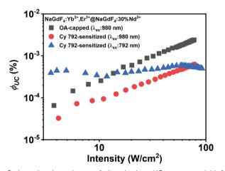
Fig. 6 Intensity dependence of the absolute UC quantum yield for NaGdF<sub>4</sub>:Yb,Er@NaGdF<sub>4</sub>:30%Nd UCNCs: OA-caped UCNCs before ligand exchange dispersed in toluene (black squares); UCNCs after ligand exchange with Cy 792 dye in CD3OD under argon and without the purification process excited using a 980 nm (red circles) and a 792 nm (blue triangles) laser.
