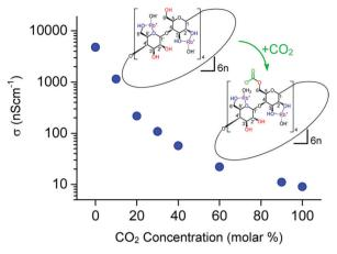
Fig. 6 Variations in the conductivity of CDMOF-2 upon CO<sub>2</sub> absorption/ desorption cycles.62
