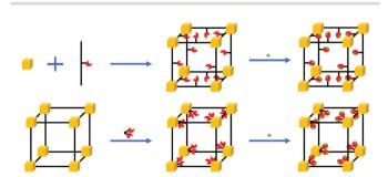
Fig. 2 A representation of synthetically modified MOFs to promote selective  $CO_2$  adsorption. Metal nodes (ion or cluster) with open metal sites (yellow), organic linker (black),  $CO_2$  molecules (green),  $CO_2$  binding sites (red).
