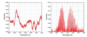
Fig. 4 Absorption spectrum of  $CO_2$  confined within HKUST-1 (left) and of reference  $CO_2$  gas inside quartz gas cell (right).<sup>49</sup>
