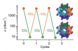
Fig. 7 Graph of the average conductivity values of CDMOF-2 as a function of the CO<sub>2</sub> concentration in N<sub>2</sub> atmosphere. The structural change of the MOF's  $\gamma$ -cyclodextrin ( $\gamma$ -CD) linker upon reaction with CO<sub>2</sub> is also shown.62
