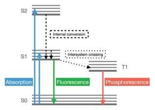
Fig. 9 Perrin-Jablonski diagram of luminescence processes.
