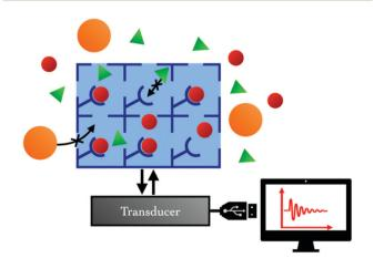
Fig. 3 The principle of MOF-based chemical sensing.
