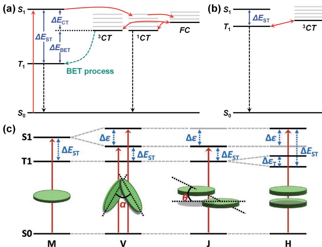
Fig. 7 (a) Schematic illustration of triplet-recombination through back electron transfer (BET) process. (b) Energy diagram with small  $\Delta E_{CT}$ ,  $\Delta E_{ST}$ , and  $\Delta E_{BET}$ . (c) Schematic energy diagram of  $S_1$  and  $T_1$  splitting according to molecular packing modes (V-type, J-type, and H-type molecular packing structures). Reproduced with permission.<sup>155</sup> Copyright 2020, WILEY-VCH.
