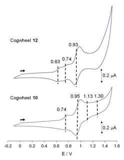
Fig. 8 Cyclic voltammograms of cogwheels 10 and 12 versus SCE ( $CH_2CI_2$ , 0.1 M  $nBu_4NPF_6$ , 25 °C, scan rate: 0.1 V s<sup>-1</sup>).
