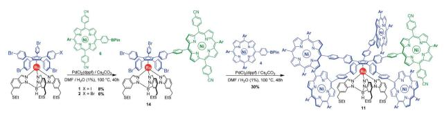
Scheme 4 Synthesis of the chemically-tagged cogwheel 11, incorporating one distinct electron-deficient porphyrinic macrocycle (in green), via sequential Suzuki–Miyaura cross-coupling reactions. Ar = 3,5-di-tert-butylphenyl.
