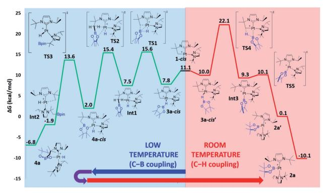
Fig. 6 Gibbs energy profile in dichloromethane for the C-B (green trace) and C-H (red trace) bond formation pathways (NHCs in cis) upon reaction between 1 and HBpin. Gibbs energies at 298 K in kcal mol<sup>-1</sup>. The Gibbs energy of 1 + HBpin has been taken as zero-energy.
