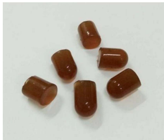
Fig. 10 The appearance of XG-g-PAA/GO composite hydrogel.
