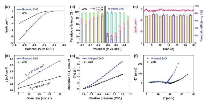
Fig. 3 The CO₂RR performance of ZnO and N-doped ZnO nanorods. (a) LSV curves, (b) FEs of CO, CH₄ and H₂ at various applied potentials, (c) stability test for N-doped ZnO nanorods at -0.7 V vs. RHE and the FE variation for CO production, (d) charging current density differences j plotted against the scan rates, (e) CO<sub>2</sub> adsorption isotherms, and (f) Nyquist plots of EIS.
