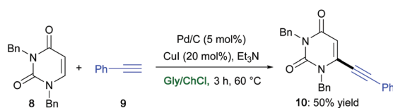
Scheme 11 Synthesis of uracil derivative 10 via a Pd-catalyzed Sonogashira cross-coupling reaction in ChCl/Gly.
