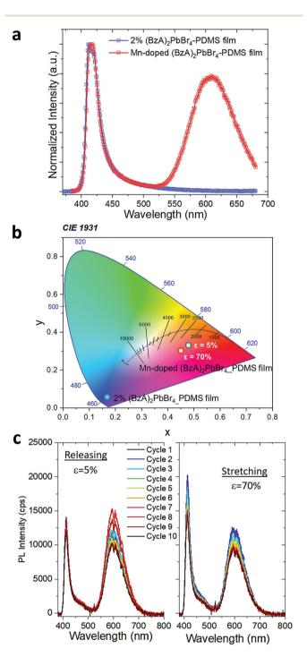
Fig. 4 (a) Emission spectrum of the Mn-doped (BzA)<sub>2</sub>PbBr<sub>4</sub>-PDMS free-standing film showing a dual emission profile. (b) CIE chromaticity coordinates of the composite films. (c) Opto-mechanical response of Mn-doped (BzA)<sub>2</sub>PbBr<sub>4</sub>-PDMS free-standing film under continuous stretch/release mechanical cycles.
