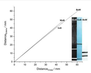
Fig. 3 Left: Steps vs. distance and steps vs. force show a strong linear correlation. Right: Crosshead vs. image analyzed distances between two marks show a strong linear correlation.
