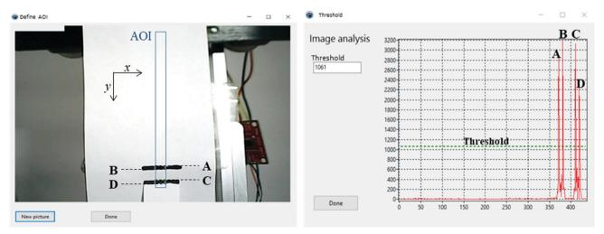
Fig. 2 Video extensometer menu with AOI (left) and defined threshold (green dashed line) for the resulting red trace (right). Graph: averaged difference values as a function of vertical (y) pixel number in AOI.
