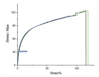
Fig. 5 Results from a PP experiment measured on the CMTT, where strain is calculated from grip-to-grip (black), extensometer (blue), and postprocessed via ImageJ (green).
