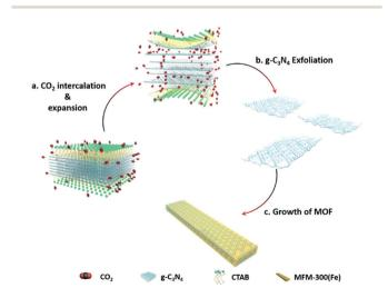
Scheme 1 Schematic illustration of scCO<sub>2</sub>-assisted exfoliation of bulk g-C<sub>3</sub>N<sub>4</sub> and the in situ synthesis of the CNNS/MFM-300(Fe) composite.
