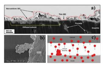
**Fig. 5** Scanning electron microscopy (SEM) image of the SEI layer in a LIB anode<sup>54</sup> (a) SEM image of a lithium dendrite<sup>55</sup> (b); schematic representation of the lithium dendrite formation process (c).
