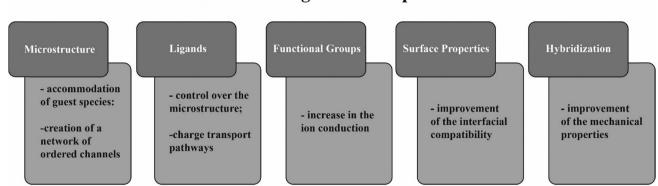
Fig. 7 Schematic representation of the main modification strategies of microporous materials and their effect in properties relevant for solid electrolytes.
