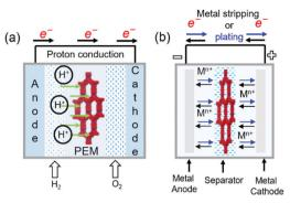
Fig. 18 Representation of working principles in (a) COFs proton conductor in polymer electrolyte membrane fuel cells (PEMFCs). (b) Metal stripping and plating through a COF based soli-state electrolyte acting as ion conductor.
