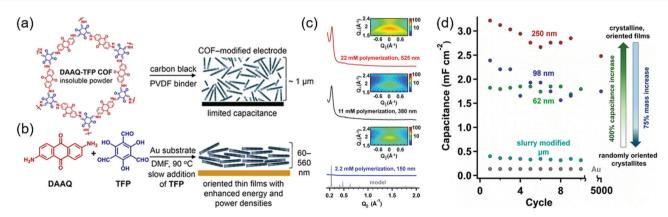
Fig. 3 Fabrication of COF thin films and pseudo-capacitor performance. (a) COF structure as 2D-layered microcrystalline powder. (b) Solvothermally grown COF thin film on Au electrodes. (c) Grazing incidence X-ray diffraction (GIXD) of COF films grown using different monomer concentrations. (d) Capacitance of COF thin films of varying thickness derived from galvanostatic charge-discharge experiments. Reproduced with permission.<sup>49</sup> Copyright 2015, American Chemical Society
