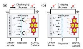
Fig. 15 Representation of working principles in COF-based Li-sulfur batteries. (a) Discharging process (b) charging process in COF-based Lisulfur batteries.
