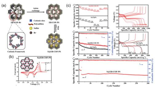
Fig. 17 Cationic COFs for trapping LiPSs in Li-sulfur battery. (a) Depiction of design, synthesis and sulfur loading in EB-COF. (b) Cyclic voltammogram of S@EB-COF-PS at increasing scan-rates. (c) Electrochemical performance of S@EB-COF-PS and S@TpPa (COF synthesized for comparison purpose) in metal-COF-sulfur battery. Reproduced with permission. 132 Copyright 2020, Wiley VCH.
