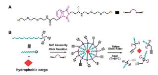
**Fig. 1** (A) Chemical structure of the novel thermoresponsive crosslinker. (B) Assembly and breakdown of temperature-responsive surface crosslinked micelle (thermo SCM). In water, the trialkyl-functionalized surfactant 2 shown at the left, readily self-assembles into a micelle structure as it encapsulates a hydrophobic cargo. Heating above 60 °C initiates the retro Diels Alder (rDA) reaction within the crosslinker, and the consequent breakdown of SCM releases the internal cargo.
