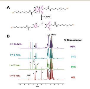
Fig. 2 (A) Schematic representation of the thermoXlinker undergoing retro-Diels-Alder (rDA) at 70 °C and yielding the decomposition products. (B)  $^1$ H NMR spectral monitoring of the rDA reaction indicating the percent dissociation of thermoXlinker ( $c_{initial} = 1.5$  mM) over time. Black arrows point to protons d and e.
