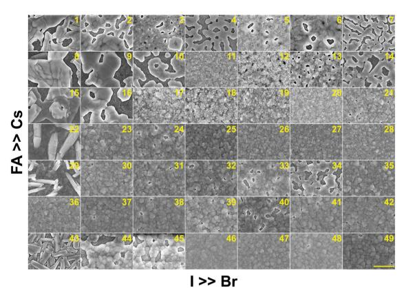
Fig. 7 Top-view SEM images of the perovskite films in the  $Cs_vFA_{1-v}Pb(Br_x|_{1-x})_3$  compositional space. The panels are arranged in the same order as in the composition matrix of Fig. 1A. The yellow scale bar on the right bottom is 1 µm.
