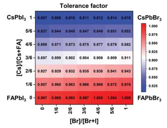
Fig. 2 Effective tolerance factor map for the  $Cs_xFA_{1-x}Pb(Br_vI_{1-v})_3$  compositional space tuned via composition engineering
