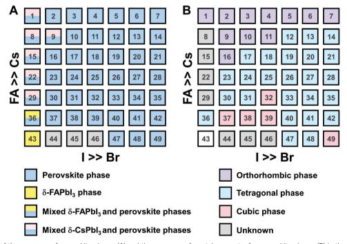
Fig. 6 Color map of the presence of perovskite phases (A) and the presence of crystal symmetry for perovskite phases (B) in the  $Cs_xFA_{1-x}Pb(Br_yI_{1-y})_3$  compositional space based on the XRD and GIWAXS data. (B) only show the crystal symmetry for the perovskite phases in (A) and the empty square for FAPbI<sub>3</sub> (No. 43) is non-perovskite phase.
