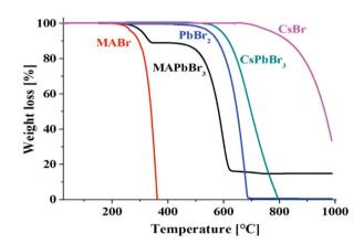
Fig. 7 Thermogravimetric analyses of MABr, MAPbBr<sub>3</sub>, PbBr<sub>2</sub>, CsPbBr<sub>3</sub>, and CsBr, showing the higher thermal stability of the inorganic perovskites compared to the hybrid organic-inorganic perovskites. Reprinted with permission from ref. 125. Copyright (2016) American Chemical Society.
