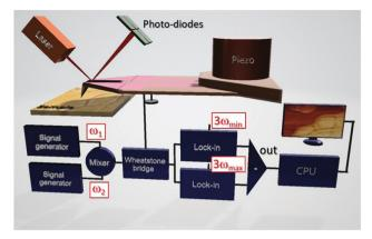
Fig. 6 Schematic illustration of extended quantitative thermal conductivity measurements by SThM applying the so-called 3ω-technique in the frequency domain. Reprinted with permission from ref. 50. Copyright (2019) American Chemical Society.
