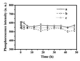
Fig. 5 Stability of the RTP intensities of (a) MPTS-ZnS QDs:Mn, (b) Mndoped ZnS QD@MIPs and (c) Mn-doped ZnS QD@ms-MIPs.
