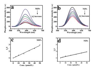
Fig. 10 (a) The RTP emission spectra of Mn-doped ZnS QD@ms-MIPs (30 mg  $L^{-1}$ ) and (b) Mn-doped ZnS QD@ms-NIPs (30 mg  $L^{-1}$ ) with the addition of different concentrations of phenol in DDW. The Stern–Volmer values for (c) Mn-doped ZnS QDs@ms-MIPs and (d) Mn-doped ZnS QDs@ms-NIPs.
