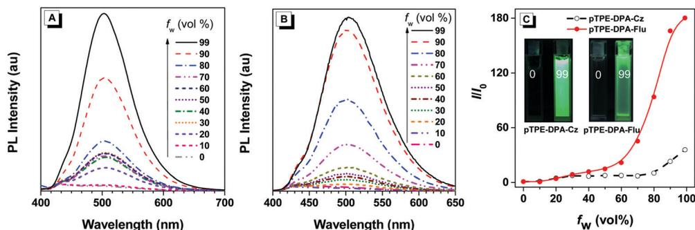
Fig. 2 PL spectra of (A) pTPE-DPA-Cz and (B) pTPE-DPA-Flu in THF/water mixtures with different water fractions ( $f_w$ ). (C) Plots of  $I/I_0$  values versus  $f_w$ .  $I_0$  is the PL intensity in pure THF. Inset: The photographs of the polymers in THF and THF/water mixtures with  $f_w$  of 99%.
