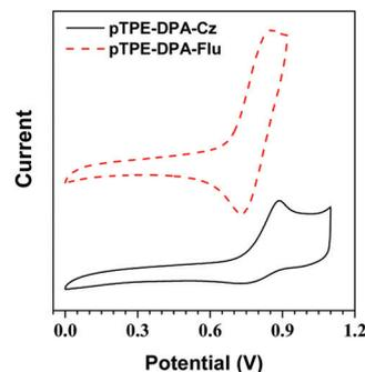
Fig. 3 Cyclic voltammograms of pTPE-DPA-Cz and pTPE-DPA-Flu measured in DCM containing 0.1 M tetra-*n*-butylammonium hexafluorophosphate. Scan rate: 100 mV s<sup>-1</sup>.
