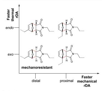
Fig. 2 Influence of the regio- and stereochemistry in the thermal and mechanochemical cycloelimination of F-M cycloadducts.83
