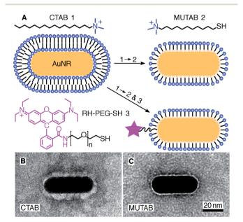
Fig. 1 (A) A gold nanorod (AuNR) coated with an adsorbed CTAB (molecule 1) bilayer is functionalized with MUTAB (molecule 2) to create a monolayer of cationic ligands covalently bound to the nanorod surface via gold—thiol bonds (top row). Alternatively, MUTAB was complemented with a rhodamine—PEG—thiol derivative (RH—PEG—SH, n=77, molecule 3) as a fluorescent label. Negative-stained TEM images of (B) CTAB-coated and (C) MUTAB-functionalized AuNRs.
