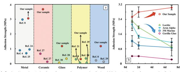
Fig. 4 Benchmarking underwater bonding performance of nanocomposite adhesives. (a) Underwater bonding of nanocomposite adhesives compared to other adhesives reported in the literature. (b) Adhesion strength of nanocomposite adhesives as a function of time used underwater in comparison with the commercial products. Lap shear joints were between aluminum substrates.
