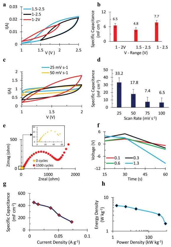
Fig. 8 For the lig-Ni-CoWO<sub>4</sub>, CV plots for different potential windows (a) and at different scan rates (c); specific capacitance variation with voltage windows (b) and scan rates (d); Nyquist plot (e); V vs. T plot (f) at varying current density (A g<sup>-1</sup>); variation of specific capacitance with current density (g); and the Ragone plot (h).
