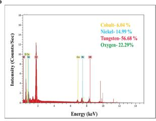
Fig. 4 EDS analysis for (a) CoWO<sub>4</sub>, and (b) Ni-CoWO<sub>4</sub> nanoparticles.
