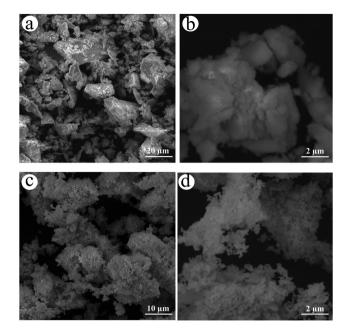
Fig. 3 SEM images for (a)  $CoWO_4$  (low magnification), (b)  $CoWO_4$  (high magnification), (c)  $Ni-CoWO_4$  (low magnification), and (d)  $Ni-CoWO_4$  (high magnification).
