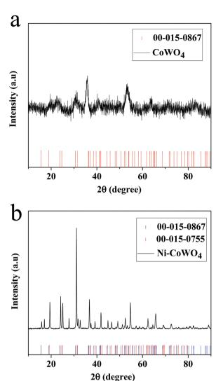
Fig. 2 XRD plots for the composite electrodes: (a) CoWO $_4$ , and (b) Ni-CoWO $_4$ .
