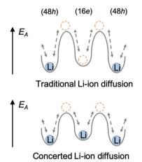
Fig. 6 Comparing traditional Li-ion diffusion (above) and the proposed concerted Li-ion diffusion (below), in which a flatter energy landscape is induced by the unique interstitial Li-ions at the 16e sites, enabling easier inter-cage jumping
