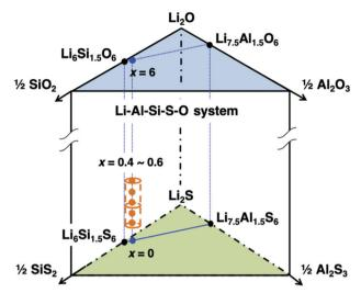
Fig. 1 Schematic composition diagram of the Li-Al-Si-S-O system (found between the pseudo-ternary Li<sub>2</sub>O-SiO<sub>2</sub>-Al<sub>2</sub>O<sub>3</sub> and Li<sub>2</sub>S-SiS<sub>2</sub>-Al<sub>2</sub>S<sub>3</sub> diagrams). The argyrodite-type phase appears in a narrow region, as indicated by a dashed cylinder. Samples with the  $Li_{6.15}Al_{0.15}Si_{1.35}S_{6-x}O_x$ (LASSO) (0.4  $\leq x \leq$  0.9) composition were synthesized.
