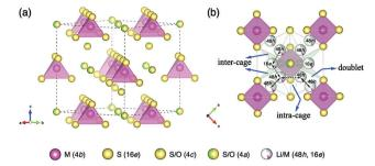
Fig. 5 (a) The  $\text{Li}_{6.15}\text{Al}_{0.15}\text{Si}_{1.35}\text{S}_{5.4}\text{O}_{0.6}$  framework with the HT-argyroditetype structure (M =  $Al_{0.1}Si_{0.9}$ ). (b) Lithium diffusion pathways, showing three types of Li migration: doublet (solid line), intra-cage (dashed line), and inter-cage (dotted line).
