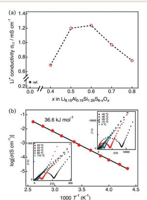
Fig. 3 (a) Lithium ion conductivity of LASSO as a function of the nominal x, as obtained by impedance spectroscopy at 25 °C. The conductivity data for x = 0 was obtained from the literature.<sup>25</sup> (b) Impedance plots for conductivity data between -45 and 110 °C (insets) and the Arrhenius plot for Li<sub>6.15</sub>Al<sub>0.15</sub>Si<sub>1.35</sub>S<sub>5.4</sub>O<sub>0.6</sub>. Conductivities were obtained by summing the grain-boundary and bulk resistances.
