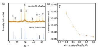
Fig. 2 (a) X-ray diffraction pattern for Li<sub>6.15</sub>Al<sub>0.15</sub>Si<sub>1.35</sub>S<sub>5.4</sub>O<sub>0.6</sub> along with the pattern of argyrodite Li<sub>7</sub>PS<sub>6</sub> (ICSD: 421130), which is indexed as the cubic argyrodite phase. (b) Lattice parameter for  $\text{Li}_{6.15} \text{Al}_{0.15} \text{Si}_{1.35} \text{S}_{6-x} \text{O}_x$  as a function of the nominal oxygen content x. The lattice data for x = 0 are taken from the literature.25
