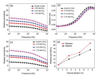
Fig. 4 Frequency dependence of (a) relative dielectric permittivity and (b) dielectric loss of BaTiO<sub>3</sub>/P(VDF-CTFE) nanocomposites with aligned BaTiO<sub>3</sub> nanowires, (c) relative dielectric permittivity of nanocomposites with random distributed BaTiO<sub>3</sub> nanowires; (d) relative dielectric permittivity of the nanocomposites as a function of volume fraction at 1 kHz.
