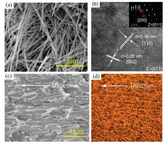
(a) SEM image of BaTiO<sub>3</sub> nanowires; (b) HRTEM image of a single BaTiO<sub>3</sub> nanowire; (c) SEM and (d) POM images of nanocomposites prepared by 3D printing with 5 vol% aligned BaTiO<sub>3</sub> nanowires.
