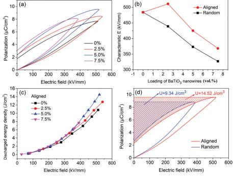
Fig. 5 (a) P-E loops and (c) discharge energy density of P(VDF-CTFE) nanocomposites filled with aligned BaTiO<sub>3</sub> nanowires; (b) breakdown strength of P(VDF-CTFE) nanocomposites as a function of BaTiO<sub>3</sub> loading; (d) comparison of maximum discharged energy density and P-E loops of P(VDF-CTFE)nanocomposites with 5.0 vol% aligned and randomly distributed BaTiO<sub>3</sub> nanowires.
