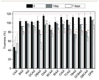
Fig. 3 Trueness values of HAAs and dalapon in tap water fortified at a concentration of 5  $\mu$ g L<sup>-1</sup> and stored at -20 °C for 7 days. Error bars indicate RSD values of n = 3 measurements.
