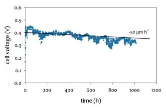
Fig. 12 A ca. 250 cm<sup>2</sup> MEA operated at 67 °C 0.4 A cm<sup>-2</sup> over 1000 h. The indicated degradation line of  $-50 \,\mu\text{V} \, \text{h}^{-1}$  holds for  $\sim 600 \, \text{h}$ . Data recorded at PO-CellTech.
