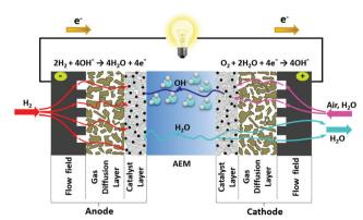
Fig. 3 Illustration of the water dynamics in operating AEMFCs – showing the water produced and consumed by the reactions, electro-osmotic drag from the cathode to anode, and back-diffusion of water from the anode to the cathode. Reproduced with permission from ref. 93
