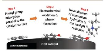
**Fig. 7** Quaternary ammonium neutralization process by electrochemical phenyl oxidation at ORR potential. The scheme is reproduced from ref. 208.
