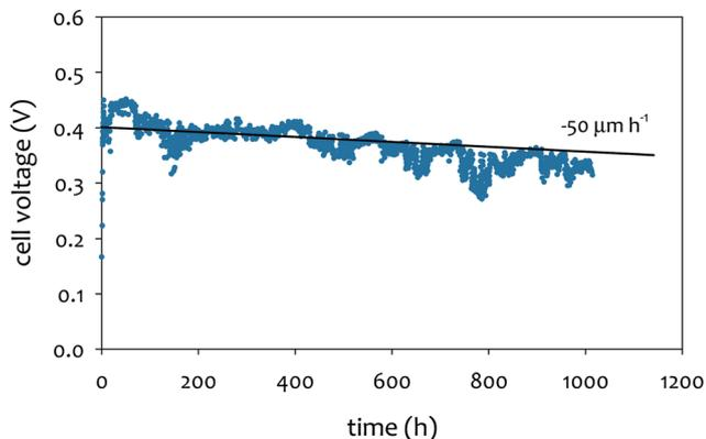
Fig. 12 A ca. 250 cm<sup>2</sup> MEA operated at 67 °C 0.4 A cm<sup>-2</sup> over 1000 h. The indicated degradation line of  $-50 \mu\text{V h}^{-1}$  holds for  $\sim 600$  h. Data recorded at PO-CellTech.
