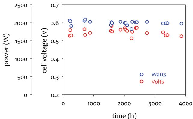
Fig. 13 Durability of AEMFC stack during intermittent operation. Reproduced data from ref. 128.
