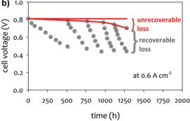
Fig. 1 (a) Fuel cell performance loss overtime in a hypothetical fuel cell system designed to deliver the power density of 1.0 W cm<sup>-2</sup>. The initial performance starts with rated power (0.76 V at 80 °C). (b) Illustration of recoverable and unrecoverable AEMFC performance loss during constant current operation mode
