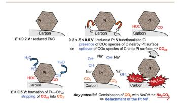
Fig. 10 Schematic representation of the processes leading to the Pt nanoparticles' detachment from their carbon support during repeated potential cycling from reducing (e.g.,  $E=0.1~\rm V~vs.~RHE$ ) to oxidizing (e.g.,  $E=1.23~\rm V~vs.~RHE$ ) conditions in MOH (M = Na, K, etc.) electrolytes with Pt/C electrocatalysts. The surface groups presented are indicative and do not pretend to be exhaustive. Freely adapted from ref. 238 with permission from Wiley.
