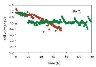
**Fig. 9** Impact of anode ionomer on AEMFC short-term stability of Pt anode catalysed MEAs. Measured the performance at 80 °C under  $\rm H_2/O_2$  (2000/300 sccm) at 147 kPa backpressure. AEM: m-TPN ( $\sim$ 35 μm thickness), ionomer: TMAOH functionalized poly(biphenylene) and TEAOH functionalized poly(biphenylene); anode: Pt/C (0.6 mg<sub>Pt</sub> cm $^{-2}$ ); cathode: Pt/C (0.6 mg<sub>Pt</sub> cm $^{-2}$ ), humidification: 80%. Reproduced from ref. 213.
