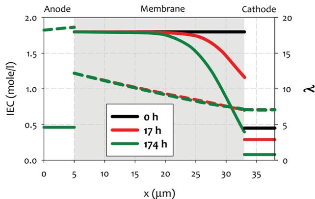
**Fig. 8** Ion exchange capacity (IEC) (full lines) and hydration number ( $\lambda$ ) (dashed lines) across the cell, at the initial stage ( $t = 0$  h) as well as at 17 h and 174 h after onset of AEMFC operation. The (constant) current density is  $0.2 \text{ A cm}^{-2}$  and the thickness of the AEM is  $28 \mu\text{m}$ . Reproduced from ref. 212.
