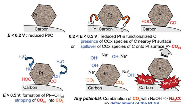
Fig. 10 Schematic representation of the processes leading to the Pt nanoparticles' detachment from their carbon support during repeated potential cycling from reducing (e.g.,  $E = 0.1 \text{ V vs. RHE}$ ) to oxidizing (e.g.,  $E = 1.23 \text{ V vs. RHE}$ ) conditions in MOH (M = Na, K, etc.) electrolytes with Pt/C electrocatalysts. The surface groups presented are indicative and do not pretend to be exhaustive. Freely adapted from ref. 238 with permission from Wiley.
