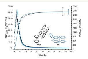
Fig. 4 Photocatalysis experiment with [12a]Br in black and the parent catalyst 13 in blue. TOF (dots) ( $H_2/Co/h$ ) and TON (lines) ( $H_2/Co$ ) formed as a function of time for 5  $\mu$ M catalyst. Experimental conditions: 10 mL solution, 0.5 mM [Ru(bpy)<sub>3</sub>]Cl<sub>2</sub>, 0.1 M NaAsc, 0.1 M TCEP, pH 5.0, 453 nm LED irradiation.
