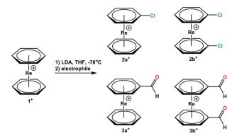
Scheme 2 Reaction scheme for the functionalization of  $[Re(\eta^6-C_6H_6)_2]$  (OTf). Reaction conditions: (1) Lithiation/deprotonation 1.5–2.5 eq. of LDA, 1.5 h, -78 °C, THF; (2) *in situ* electrophilic attack 5 h, -78 °C, THF; electrophiles:  $C_2Cl_6$  and DMF. Combined yields: (63.1% for  $2a^+$ ,  $2b^+$  and  $2c^+$ ; 43.2% for  $3a^+$  and  $3b^+$ ).
