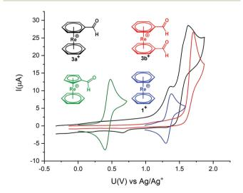
Fig. 1 Cyclovoltammogram of complexes  $1^+$  (blue),  $3a^+$  (black),  $3b^+$  (red) and mixed sandwich arene-Cp aldehyde (green); acetonitrile, 0.1 M [TBA][PF $_6$ ] (electrolyte), glassy carbon working electrode (i.d. = 3 mm), Pt auxiliary electrode, and Ag/AgCl reference electrode, analyte concentrations 1 mM, voltage step: 6 mV, sweep rate: 0.1 V s $^{-1}$ .
