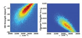
Fig. 9 Equilibrium distributions of OH stretch frequency versus HB strength, as quantified by the  $\Delta E_{\text{CT}}$  terms (left) and the associated charge-transfer terms ( $\Delta Q_{\text{CT}}$  in units of elementary charge, right). The frequencies of the OH modes were calculated using a wavelet-based time-series analysis. 18,50,51 Reproduced from ref. 18/CC BY.
