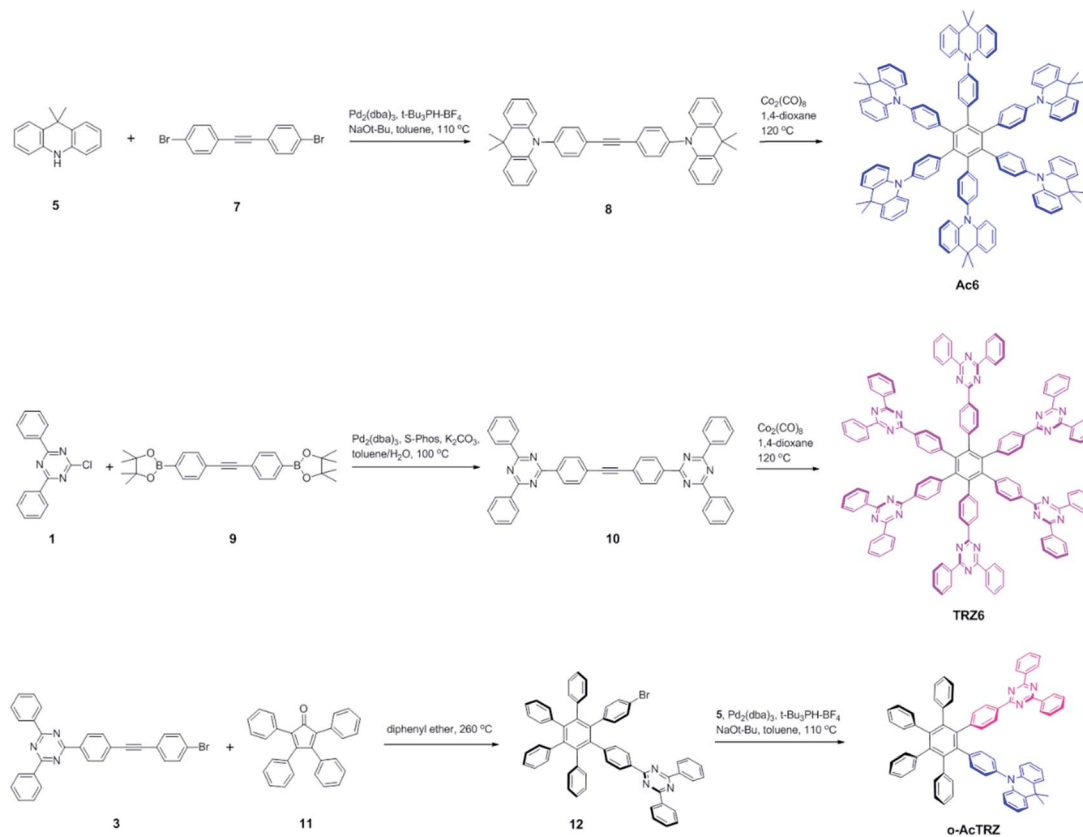
Scheme 2 Synthesis of the control compounds Ac6, TRZ6 and o -AcTRZ.
