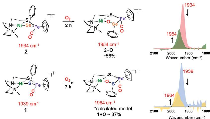
Fig. 4 Reactions of **1** and **2** in the presence of 1 atm O<sub>2</sub> in CH<sub>2</sub>Cl<sub>2</sub> at 22 °C; conversions determined by ν(CO) analysis.
