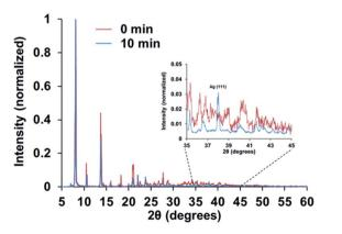
Fig. 5 XRD diffraction pattern for complexes 2 and 2H, before and after exposure to cold hydrogen plasma, respectively. The inset legends indicate the time period of exposure to the hydrogen plasma.
