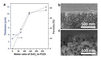
Fig. 6 Phenolic membranes prepared at different molar ratios of  $ZnCl_2$  to P123. (a) Thickness and porosity; (b, c) the cross-sectional SEM images detailing the morphology near the top surface of the membrane prepared at the molar ratios of (b) 70 and (c) 280.
