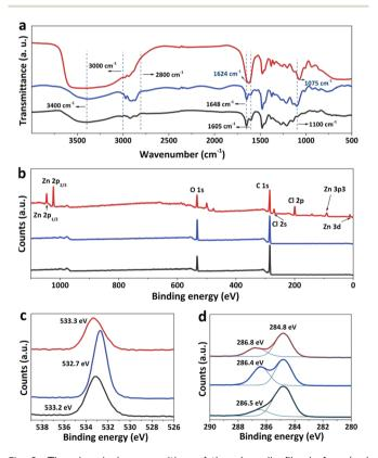
Fig. 2 The chemical composition of the phenolic film before (red curve) and after soaking in water (blue curve) or  $H_2SO_4$  (black curve). (a) IR spectra, (b) wide-scan XPS spectra, and the corresponding enlarged spectra of (c) O and (d) C.
