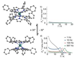
Fig. 14 Crystal structure of 39 (top) and 40 (bottom) with their associated out-of-phase magnetic susceptibility contributions. Colour code: terbium: turquoise and hydrogen: light pink. Adapted from ref. 106.
