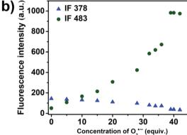
Fig. 1 (a) Changes in fluorescence emission intensity of **HMBT-LW** (5 μM) with increasing additions of  $O_2^{\bullet-}$  (from 0 to 42 equiv.) in PBS buffer solution (10 mM, V/V, DMSO/PBS = 1/1, pH = 7.4) after 3 min. (b) Emission at 378 and 483 nm of **HMBT-LW** (5 μM) with increasing addition of  $O_2^{\bullet-}$  (from 0 to 42 equiv.) in PBS buffer solution (10 mM, V/V, DMSO/PBS = 1/1, pH = 7.4) after 3 min.  $\lambda_{ex}$  = 310 nm. Slit widths: ex = 8 nm, em = 5 nm.
