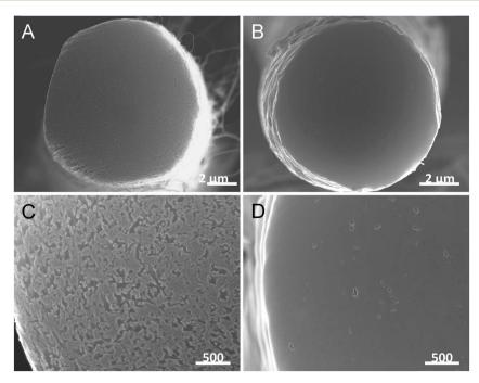
Fig. 2 The SEM images of the cross-section of a twisted carbon nanotube yarn before (A and C) and after (B and D) wax infiltration. Pores shown in the high magnification image of the neat yarn (C) are not visible in the corresponding image of the wax hybrid yarn (D). This figure has been reproduced from ref. 4 with permission from AAAS
