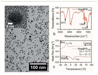
Fig. 1 (a) TEM image, the inset shoes HR-TEM image of a freestanding NP. (b) FTIR analysis and (c) DSC heat flow analysis of Mag@PB $_{1000}$  nanoparticles.
