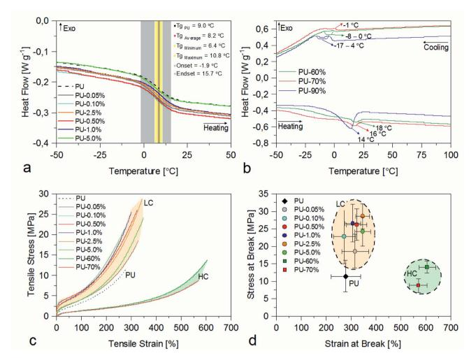
Fig. 3 (a) DSC heat flow curves for low concentration nanocomposites compositions and (b) for the highly concentrated Mag@PB<sub>1000</sub>/PU nanocomposites; (c) tensile stress–strain curves and (d) break points of the tensile test of Mag@PB<sub>1000</sub>/PU nanocomposites.
