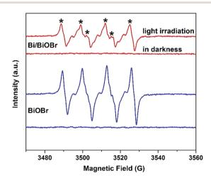
Fig. 9 ESR spectra of the as-synthesized Bi/BiOBr and BiOBr samples for  ${\rm DMPO-\cdot O_2}^-.$
