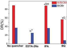
Fig. 8 Trapping experiment of active species during the photocatalytic reaction with visible light irradiation: EDTA-2Na as a scavenger for holes (h<sup>+</sup>); IPA (iso-propanol) as a scavenger for hydroxyl radicals ( $\cdot$ OH); BQ (1,4-benzoquinone) as a scavenger for superoxide radicals ( $\cdot$ O<sub>2</sub><sup>-</sup>).
