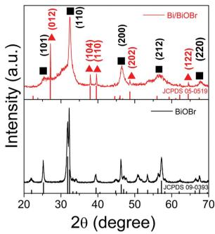
Fig. 1 XRD patterns of the Bi/BiOBr and BiOBr samples.
