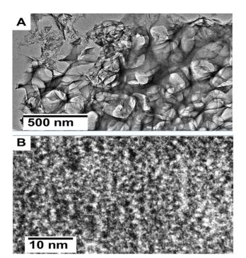
Fig. 2 (A) TEM and (B) HRTEM images of carbon nanosheets prepared from tal palm leaves at  $850\,^{\circ}$ C.
