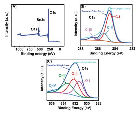
(A) XPS survey spectrum, (B) C1s and (C) O1s deconvoluted XPS spectra of the porous carbon nanosheets prepared from tal palm leaves.
