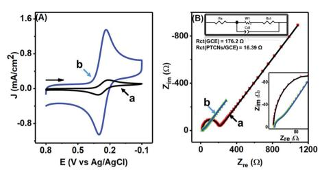
Fig. 6 (A) CVs and (B) EIS spectra of 5.0 mM K<sub>3</sub>[Fe(CN)<sub>6</sub>] in 1.0 M KCl at the GCE (a) and at the PTPCNs/GCE (b). The upper left side of (B) shows the Randel circuit, whereas the lower left inset shows the magnified EIS of the PTPCNs/GCE
