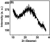
Fig. 3 (A) Raman and (B) XRD spectra of carbon nanosheets prepared from tal palm leaves.
