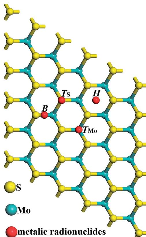
Fig. 1 Schematic diagram of the possible adsorption sites of a metallic radionuclide on monolayer  $\text{MoS}_2$ , and glaucous, yellow, and red balls represent Mo atoms, S atoms, and metallic radionuclides, respectively.
