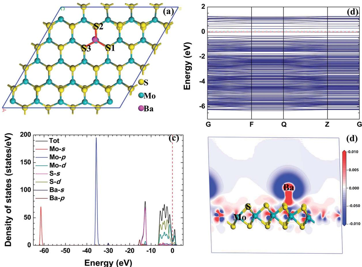
Fig. 5 The relaxed configuration, band structure (from  $-10$  eV to  $5$  eV), density of states, and electron density difference of the radionuclide Ba adsorbed on monolayer  $\text{MoS}_2$  with the initial configuration B.
