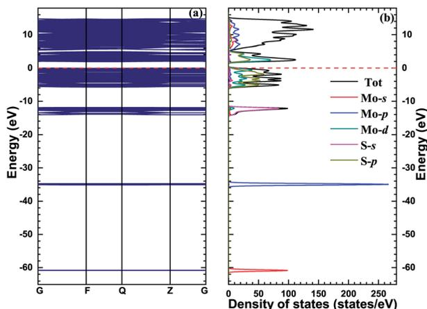
Fig. 2 The band structure (a) and density of states (b) of monolayer MoS<sub>2</sub>, and the red dashed lines stand for the Fermi level.
