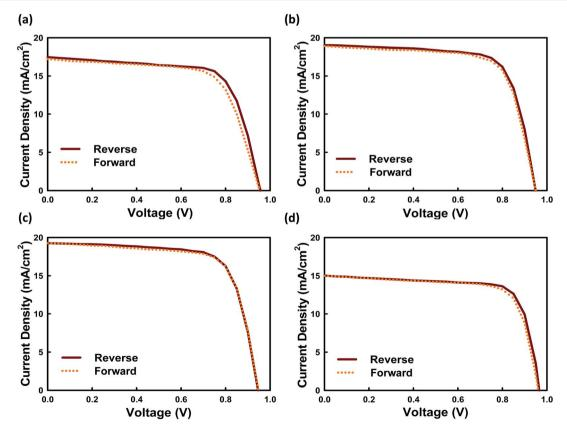
Fig. 7 J-V plots for perovskite solar cells (a) without PS, (b) with 1.5 wt% PS, (c) with 3.0 wt% PS, and (d) with 4.5 wt% PS under one sun conditions (100 mW cm<sup>-2</sup>, AM1.5G). The scan rate for both scans is 10 mV s<sup>-1</sup>.
