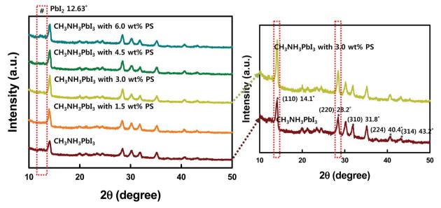
XRD diffraction patterns of CH<sub>3</sub>NH<sub>3</sub>Pbl<sub>3</sub> thin films spin-coated on glass with and without PS (1.5, 3.0, 4.5, and 6.0 wt%).
