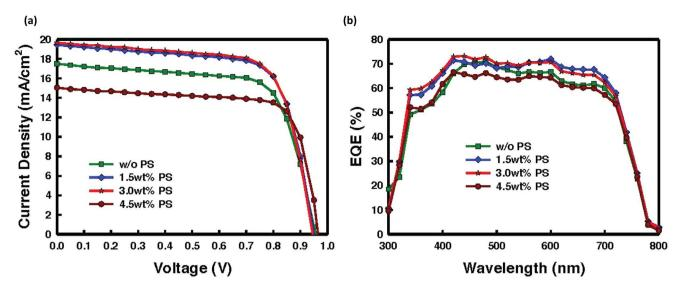
Fig. 2 Device performance of perovskite solar cells with different concentrations of polystyrene (ITO/PEDOT:PSS/CH<sub>3</sub>NH<sub>3</sub>PbI<sub>3</sub> (without or with 1.5, 3.0, 4.5 wt% PS)/PC<sub>60</sub>BM/Al). (a) J-V characteristics under one sun condition (100 mW cm<sup>-2</sup>, AM1.5G) and (b) external quantum efficiency (EQE) spectra of perovskite solar cells.
