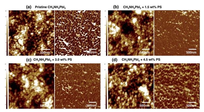
Fig. 3 Surface properties of thin films used in this work. The (a-d left panels) atomic force microscopy (AFM) and (a-d right panels) conductive AFM (cAFM) images of CH<sub>7</sub>NH<sub>7</sub>Pbl<sub>7</sub> perovskite thin film with different concentrations of polystyrene on the ITO/PEDOT:PSS layer.
