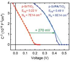
Fig. 5 Mott-Schottky analysis of p-Si/TiO<sub>2</sub> and p-Si/Al<sub>2</sub>O<sub>3</sub>/PA/TiO<sub>2</sub> PV cells obtained from impedance measurements in the dark. Experimental and fitting details are given in the ESI.† The measured doping densities match with the resistivity data provided by the manufacturer.
