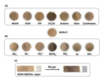
Fig. 6 Chemochromism of NION-Cl. (a) Solvochromism in CH<sub>3</sub>CN, (b) anionochromism toward N(CN)<sub>2</sub><sup>-</sup> anion, and (c) vapochromism towards NH<sub>3</sub>.
