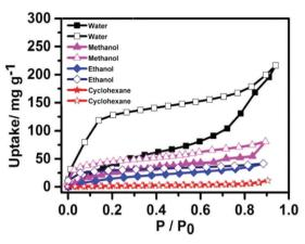
Fig. 2 Sorption isotherms of NION-Cl toward different vapors at 298 K. Solid symbols for the adsorption branch and hollow ones for the desorption branch.
