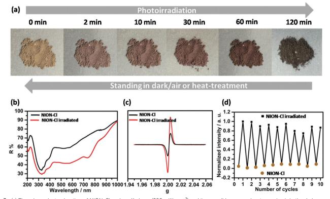
Fig. 3 (a) Time dependent coloration of NION-Cl under a Xe lamp (200 mW cm<sup>-2</sup>) and its reversible process by storage in air in the dark, a process that can be accelerated by thermal-treatment. (b) The UV-Vis diffuse reflectance spectra and (c) the ESR signal before and after photoirradiation. (d) Absorbance at  $\lambda$  = 740 nm in repeated coloring and bleaching cycles.
