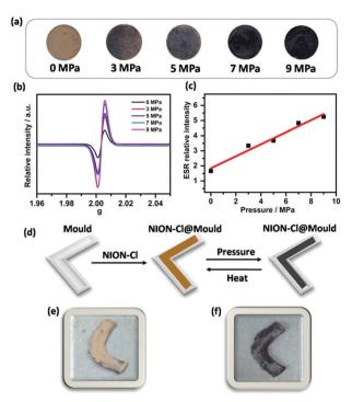
(a) Pressure dependent coloration of a NION-Cl disk. (b) ESR signals for the corresponding disk. (c) Plot of ESR intensity vs. external pressure. (d-f) Schematic illustration and real samples of the mould-assisted casting method to show the "pressure memory" effect of NION-Cl.
