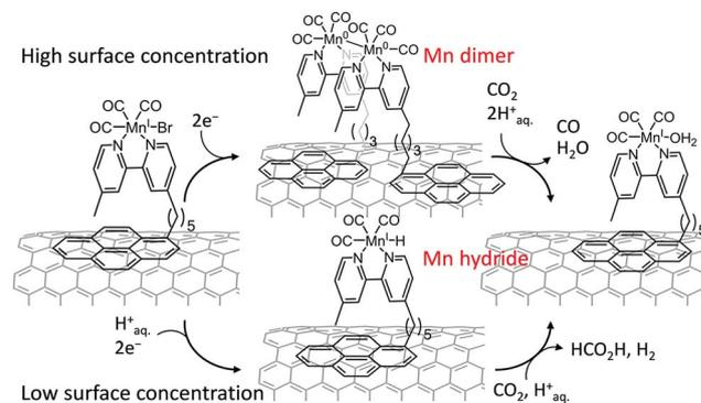
**Scheme 10** Two-electron reduction of  $\text{CO}_2$  to  $\text{CO}$  vs.  $\text{HCOOH}$  with the  $[\text{MnBr}(2,2'\text{-bipyridine})(\text{CO})_3]$  complex anchored to a carbon nanotube electrode *via* a pyrene unit depending on the surface concentration. Reprinted with permission from ref. 134. Copyright 2017, American Chemical Society.
