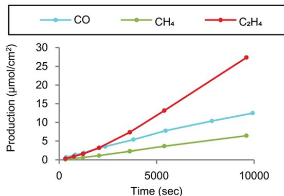
Fig. 12 Products derived from CO<sub>2</sub> electrochemical reduction by crystalline CuPc/C at  $-1.6$  V vs. Ag/AgCl in a two-compartment H-cell. Reprinted with permission from ref. 148. Copyright 2017, American Chemical Society.
