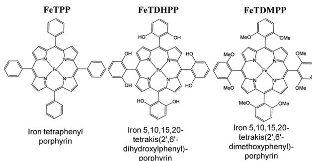
Fig. 1 Iron tetraphenylporphyrin derivatives used for electrocatalytic reduction of  $\text{CO}_2$  to CO. Reprinted with permission from ref. 86. Copyright 2012, The American Association for the Advancement of Science.
