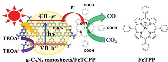
Scheme 15 Photocatalytic reduction of CO<sub>2</sub> to CO with TEOA using g-C<sub>3</sub>N<sub>4</sub> nanosheets/FeTCPP (g-C<sub>3</sub>N<sub>4</sub>/FeTCPP). Reprinted with permission from ref. 170. Copyright 2018, Elsevier.
