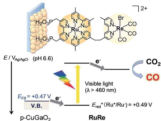
**Scheme 16** Schematic illustration for the photocatalytic reduction of CO<sub>2</sub> to CO with the RuRe/CuGaO<sub>2</sub> electrode. Reprinted with permission from ref. 173. Copyright 2017, Royal Society of Chemistry.
