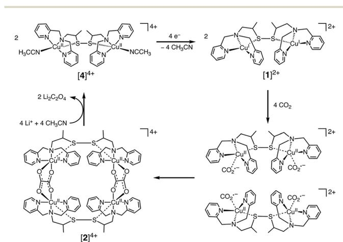
Scheme 1 Catalytic one-electron reduction of  $\text{CO}_2$  to oxalate with a dinuclear copper(I) complex ( $[\mathbf{1}]^{2+}$ ). Reprinted with permission from ref. 78. Copyright 2010, The American Association for the Advancement of Science.
