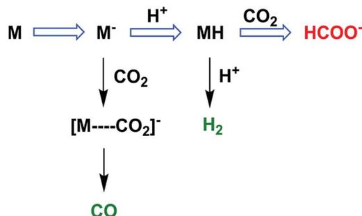
Scheme 7 The reaction pathway of two-electron reduction of CO<sub>2</sub> with a metal complex (M) to produce HCOO<sup>-</sup> or CO. Reprinted with permission from ref. 125. Copyright 2017, American Chemical Society.
