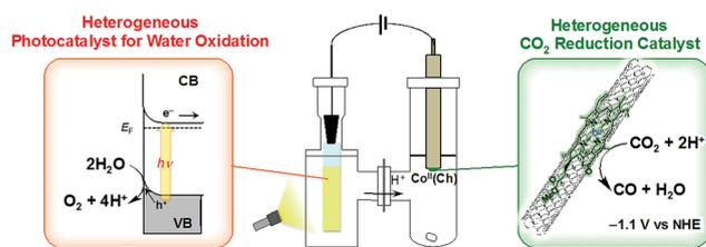
Fig. 14 Schematic illustration of a photoelectrochemical cell composed of an FeO(OH)/BiVO<sub>4</sub>/FTO photoanode for the photocatalytic oxidation of water to O<sub>2</sub> and a Co<sup>II</sup>(Ch)/MWCNT cathode for the catalytic reduction of CO<sub>2</sub> to CO. Cathode and anode compartments are separated by a Nafion membrane. Reprinted with permission from ref. 172. Copyright 2017, American Chemical Society.
