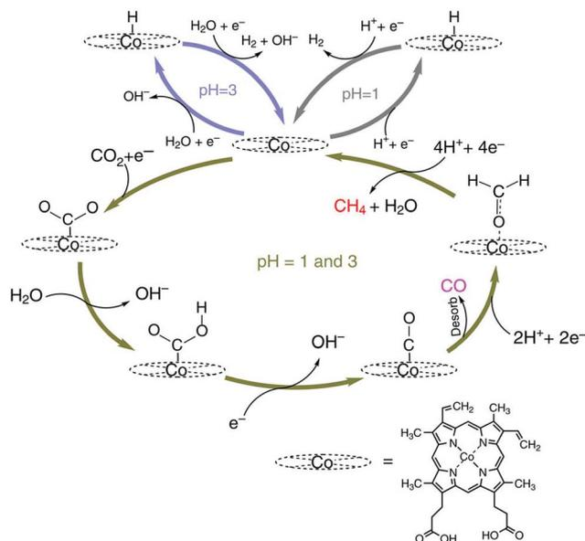
Scheme 12 Catalytic cycle for two electron reduction of CO<sub>2</sub> to CO and further reduction to CH<sub>4</sub> with a Co protoporphyrin molecular catalyst (CoPP) immobilized onto a pyrolytic graphite (PG) electrode (CoPP-PG). Reprinted with permission from ref. 147. Copyright 2015, Nature Publishing Group.
