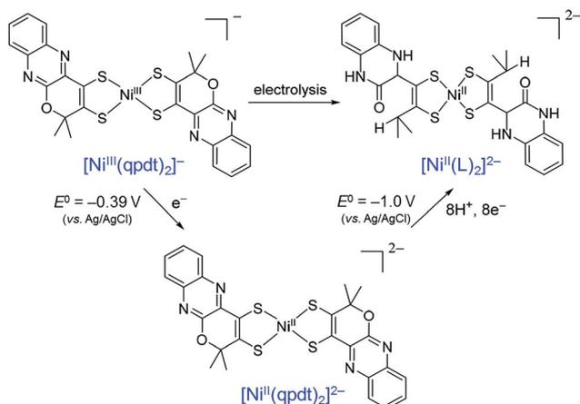
Scheme 11 Electrochemical reduction of  $[\text{Ni}(\text{qpdt})_2]^-$ , followed by the subsequent pyran ring opening to produce the real catalyst ( $[\text{Ni}^{\text{II}}(\text{L})_2]^{2-}$ ; L is a pyran ring-opened ligand produced from  $\text{qpdt}^{2-}$  by electrolysis) during electrolysis. Reprinted with permission from ref. 138. Copyright 2018, American Chemical Society.
