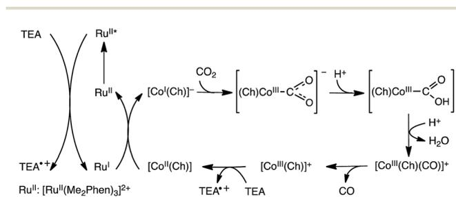
Scheme 13 Photocatalytic cycle for two-electron reduction of CO<sub>2</sub> to CO with a cobalt(II) chlorin complex (Co<sup>II</sup>(Ch)) adsorbed on multi-walled carbon nanotubes (Co<sup>II</sup>(Ch)/MWCNTs). Reprinted with permission from ref. 150. Copyright 2016, Royal Society of Chemistry.
