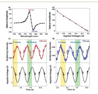
Fig. 3 (a) Scattering intensity amplitude of a single AuNR under the monochromatic illumination of different wavelengths. (b) Plot depicting the linear relationship between the applied voltages and scattering intensity amplitude. As a result of the modulating potential, original scattering intensity curves exhibit out-of-phase and in-phase responses under the illumination of (c) 740 and (d) 775 nm, respectively
