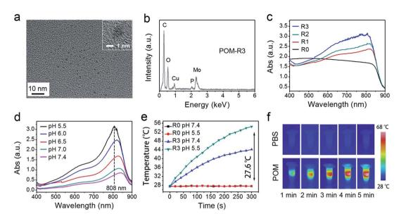
Fig. 1 TEM image (the inset shows the corresponding high resolution image) (a) and the EDS spectrum (b) of the POM-R3 cluster. UV-vis absorption spectra of POM solutions at varied reduction states (c) and the POM-R3 solution at varied pHs (d). Photothermal heating curves of POM-R0 and POM-R3 solutions at pH 5.5 and pH 7.4 (e), and photothermal heating images (f) of POM-R3 (pH 5.5) and PBS buffer solutions under 808 nm laser irradiation (0.72 W cm<sup>-2</sup>).
