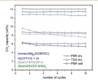
Fig. 3 CO<sub>2</sub> capture of polyamines impregnated on bulk MOFs compared with MOF/SiO2 under simulated flue gas conditions in a PBR.
