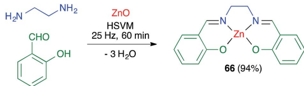
Scheme 46 Mechanochemical synthesis of a zinc-salen complex.
